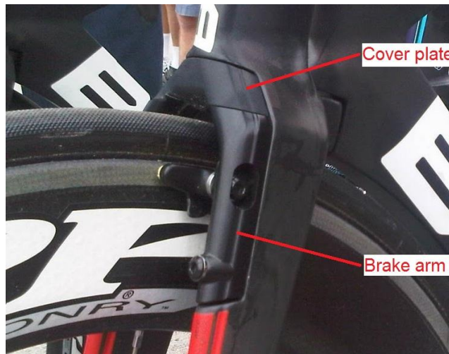
Figure 55: Brake integrated with the fork and fitted with a cover
