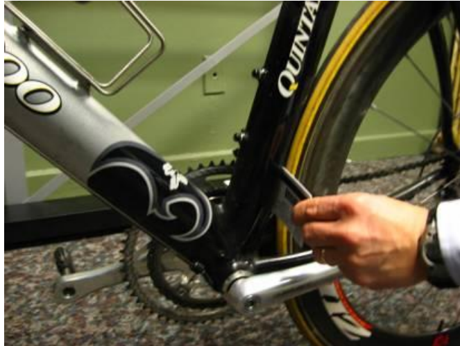
Figure 60: Insertion of a credit card between the wheel and frame to check that a fairing is not present
