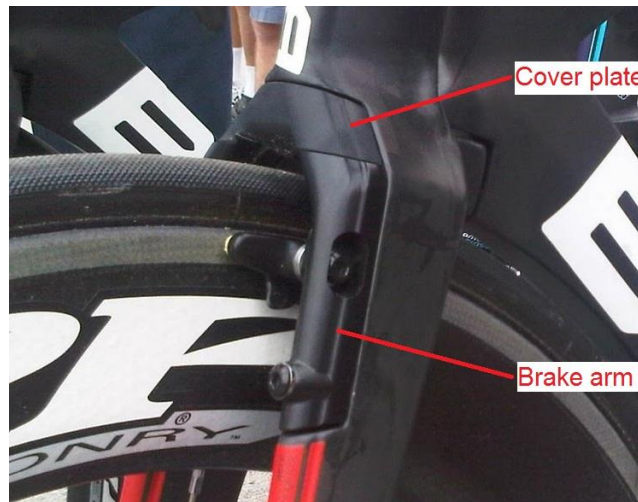
Figure 53: Brake integrated with the fork and fitted with a cover
