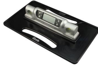
Figure 6: Official measuring device to check saddle inclination
